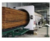
Process control for thermal modification of wood.
